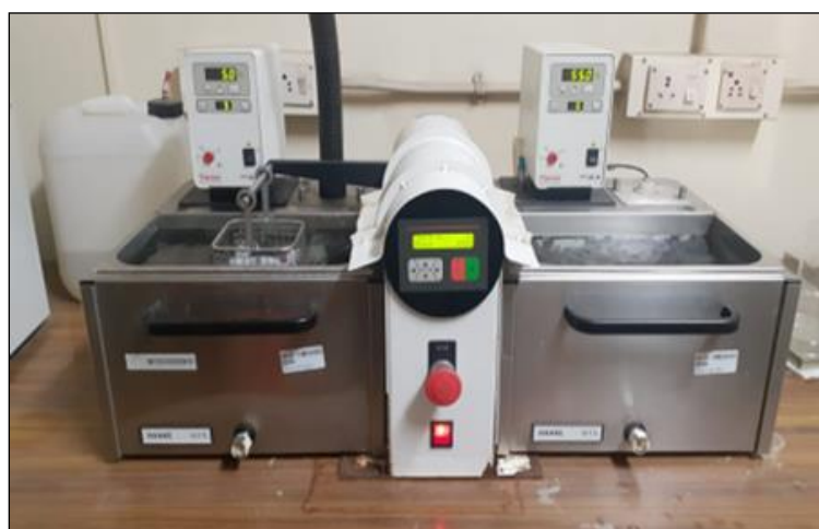
Fig 5: WILEYTEC Thermocycler with cooling system HAAKE EK 30
