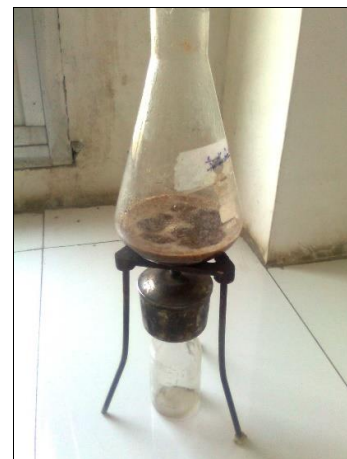
Picture 1: Image showing preparation of extract of clove powder in distilled water
