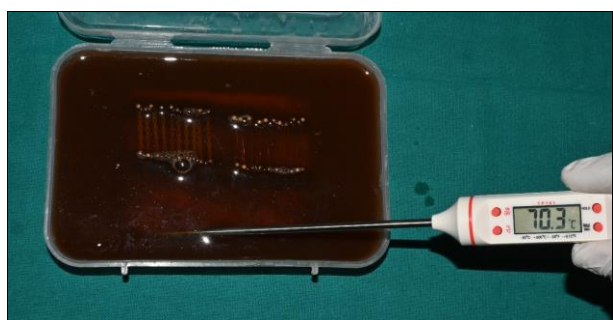
Fig 3: slab submerged in Hot Tea at a temperature of 70°C ± 1°C Group 3: The slab was submerged in Cold Drink at a temperature of 10°C ± 1°C (figure 4)
