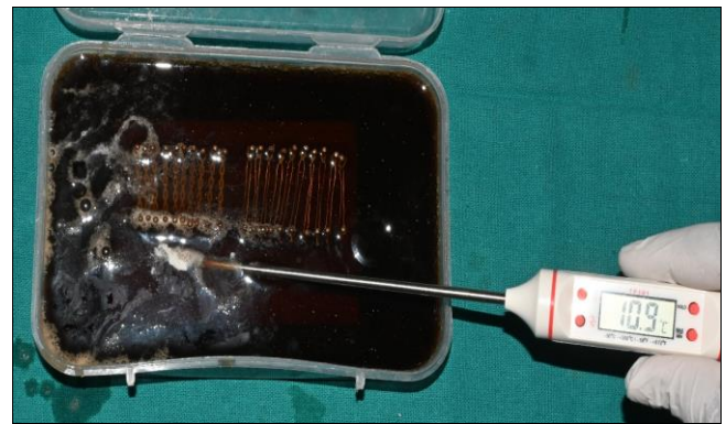
Fig 4: slab submerged in Cold Drink at a temperature of 10°C ± 1°C
