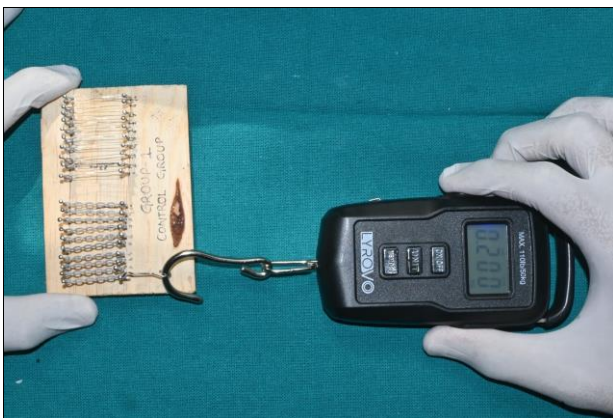
Fig 2: Measuring gauge recording at initial force of 200 grams.
