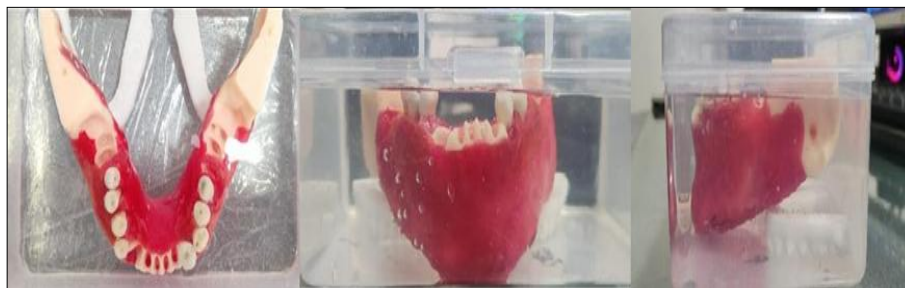
Fig 6: Top view (a), front view (b), and side view (c) of jaw covered with pink wax and placed in water to simulate soft tissue
