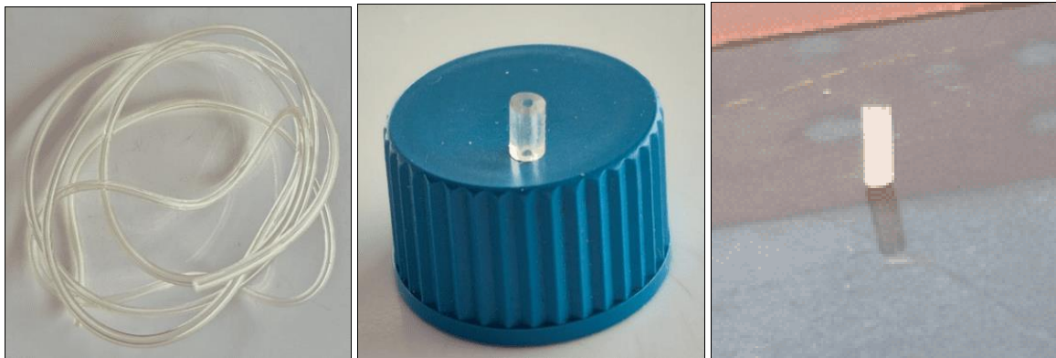
Fig 2: Fabrication of resin tubes 2 mm high and 0.8 mm in diameter using Tygon
