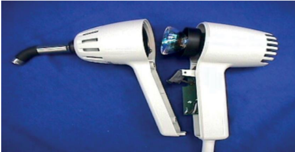
Fig 3: Internal components of a typical QTH curing light
