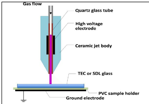
Fig 2: Atmospheric Pressure Plasma Jet
