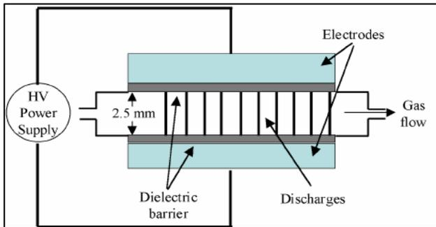
Fig 1: Dielectric Barrier Discharge
